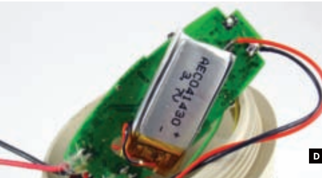
Fig. B: The telephone handset, disassembled.
